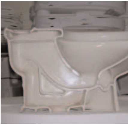
Internal parts of a bench bowl casting with mould sections in the background.
